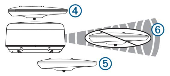
• The compass should not be mounted directly in the path of the radar 6.
