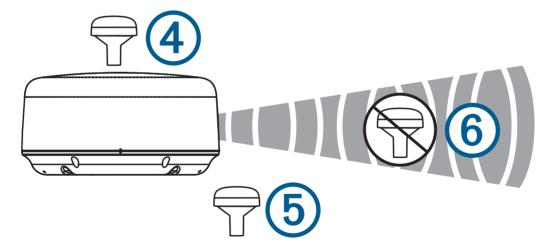
The antenna should not be mounted directly in the path of the radar  $\bigcirc$ .
